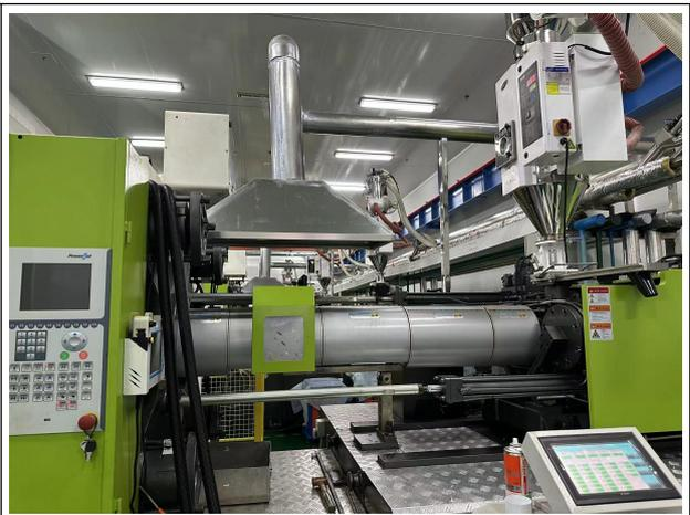
图2 产气点处加设集气罩
